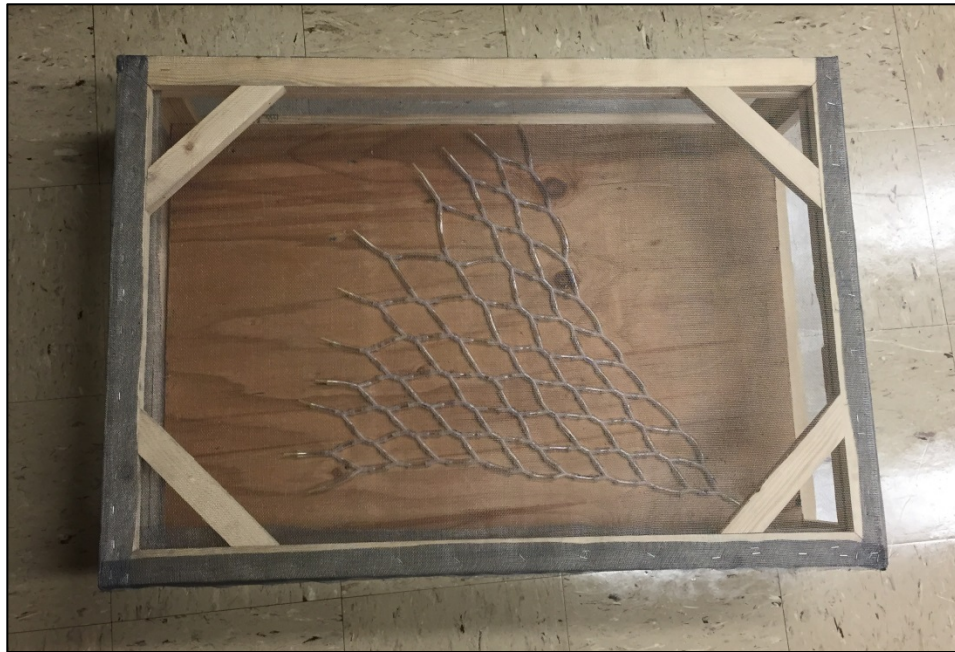
Figure 2: The Y-maze contained within the Faraday cage
