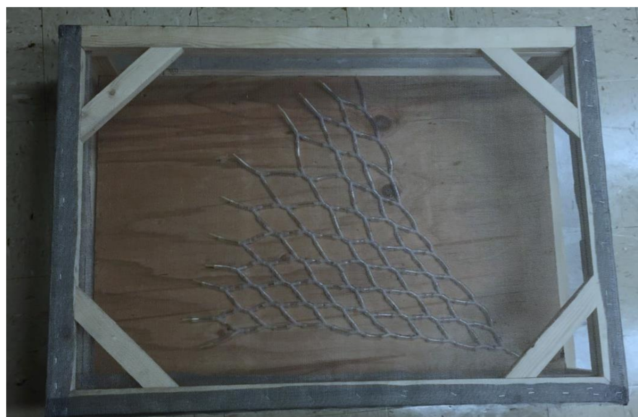
Figure 1: Photo of the Y-maze inside the Faraday cage. The Faraday cage blocks radiofrequency fields which may affect directional choices of the flies.
