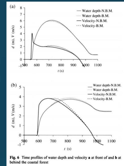
Fig. 6 Time profiles of water depth and velocity a at front of and b at behind the coastal forest
